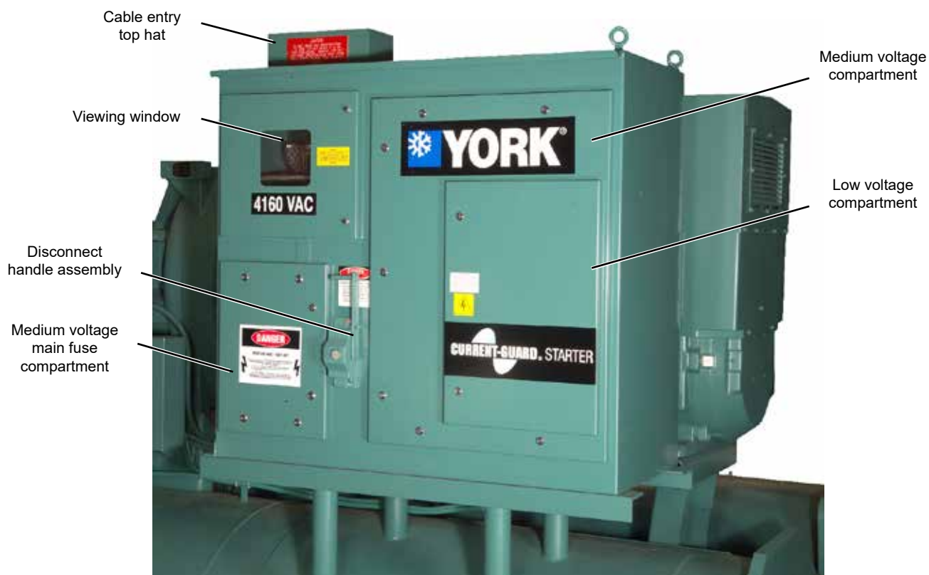
Figure 1 - Medium Voltage solid state starter – front view, exterior
