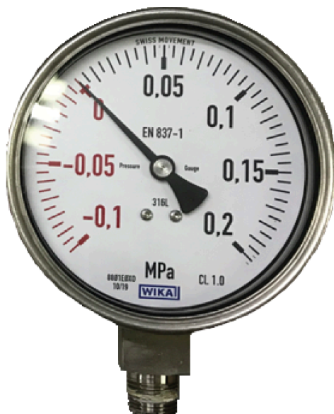
Figure 49: Compound gauge for generator
