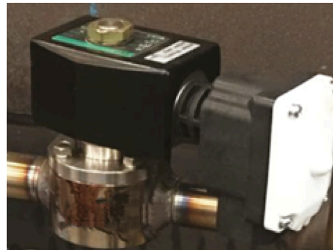
Figure 21: Solenoid valve for purge and blow pump
