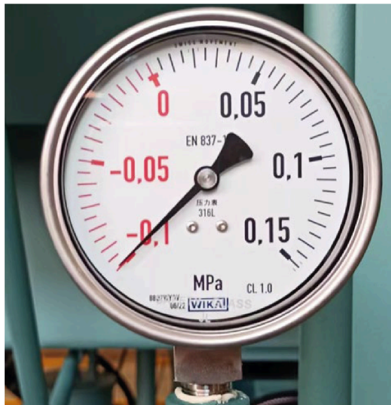
Figure 50: Compound gauge for purge line
