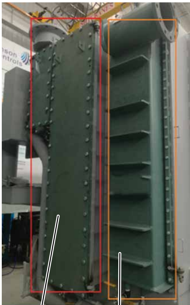
Marine Type Waterbox Compact Type Waterbox FIGURE 8 - MARINE TYPE AND COMPACT TYPE WATERBOX
