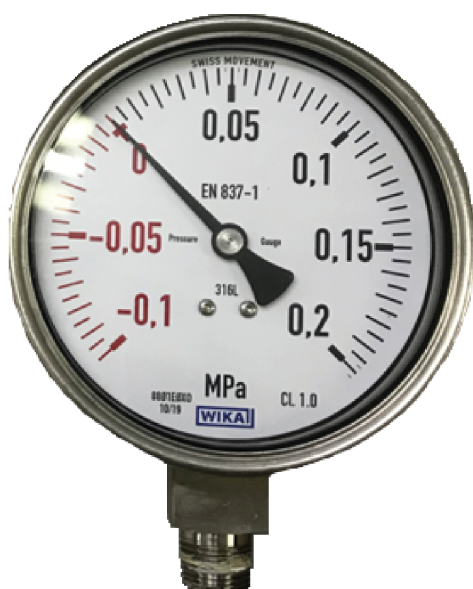
Figure 36: Compound gauge for generator
