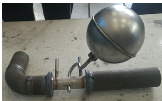
Figure 20: Refrigerant water float ball valve
